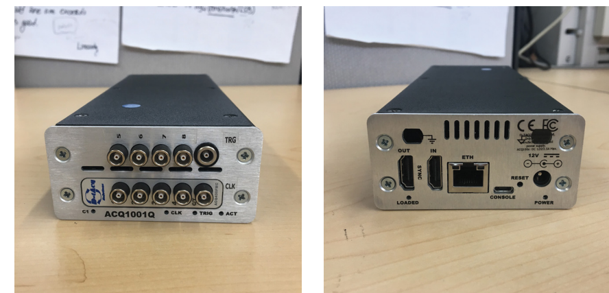
Figure 4- View of the front panel (left) and rear panel (right) of the ACQ1001-FMC digitizer
